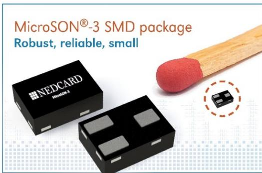
MicroSON®-3 is small and very thin, yet robust enough to withstand harsh industrial processes and high temperatures. It is a near chip scale plastic encapsulated package with a copper lead frame substrate. The leadless package makes electrical contact by soldering the bottom surface terminals to the PCB. The small size of the MicroSON®-3 design makes it a perfect package for leading RAIN RFID tag chips.
