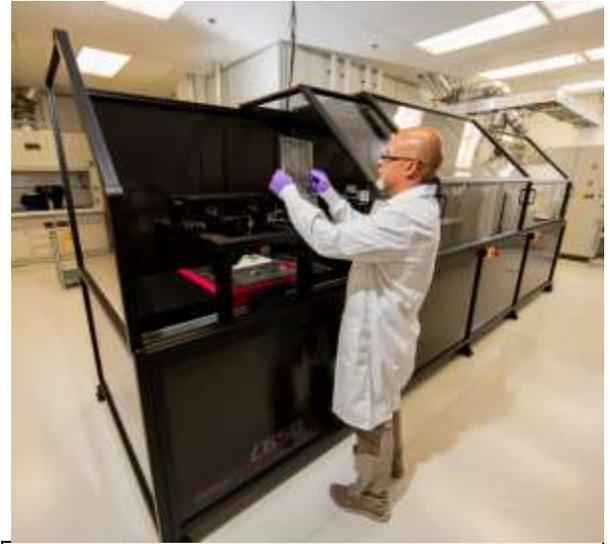
An NSM *Challenger 650* system with multiple slot-die, flexo, and gravure coating/printing stations.
