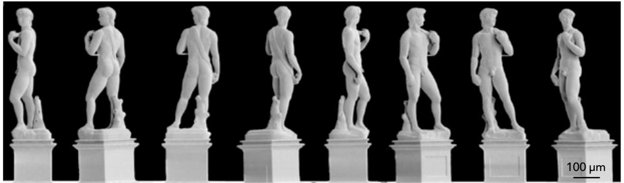
**TINY DAVID.** With the FluidFM  $\mu\text{3D}$ printer in microscale and with copper additively manufactured David from different perspectives.
