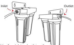
• Disconnect the 1/4" tubing from inlet and outlet on the pre-filter housing by pressing the collar in and then pulling on the tube to release (as shown below)
