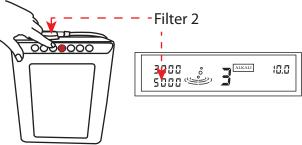
After changing the second filter, press and hold the **"FILTER 2"** button for 10 seconds. You will hear 2 beeps and the filter counter indicator will reset to 5000.
