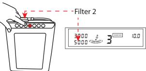
After changing the second filter, press and hold the "FILTER 2" button for 10 seconds. You will hear 2 beeps and the filter counter indicator will reset to 5000.
