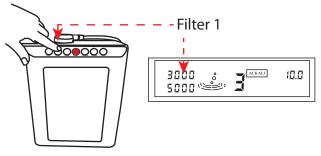
After changing the first filter, press and hold the "FILTER 1" button for 10 seconds. You will hear 2 beeps and the filter counter indicator will reset to 3000.
