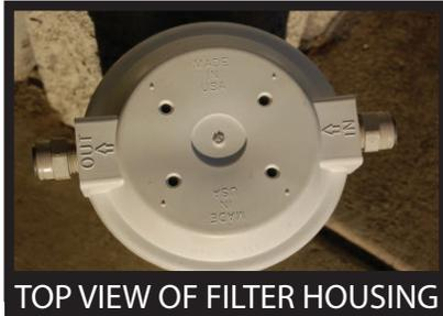
3. The tubing coming from the Reverse Osmosis Post Filter connector needs to be inserted into the side of the housing marked "IN". Firmly press the tubing into the filter-housing cap. You will feel the tubing stop when it is fully inserted. Pull on the tubing gently to ensure that it does not come out and a good connection was made.
