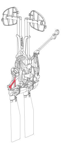
If in the forward position, pull the reverse tendon (RED) gently such that the drive rotates only half way or 90°.
