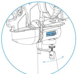
Make sure the line is away from the roll pin on <u>both sides</u> of the quadrant to avoid damaging the line with the Wrist Pin.
