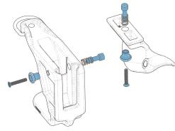
2. Grip the pin end with a pair of pliers and tighten down the screw to complete the assembly.
