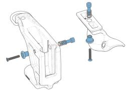
2. Grip the pin end with a pair of pliers and tighten down the screw to complete the assembly.
