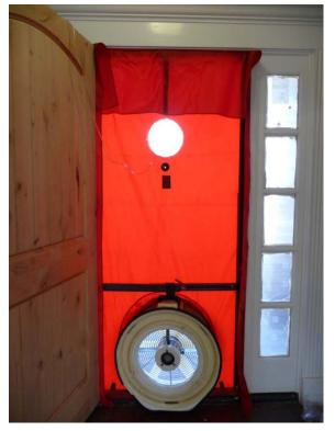
The tester measures the cubic feet of the living space (including tray ceilings!). He keeps the vents sealed, closes all doors and windows, and makes sure there is water in all the drains. He then turns on the fan in the red door, which draws air out of the inside of the house.
