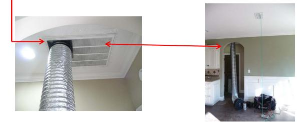
The blower door test reveals the integrity of all the openings into the interior living area: windows, doors, electrical outlets, light fixtures, air vents, boot sealants – anything that breaks the solid surface.
