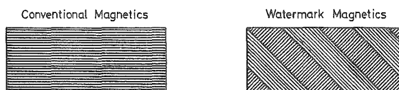
Fig. 7.4 Arrangement of 'Watermark' particles
