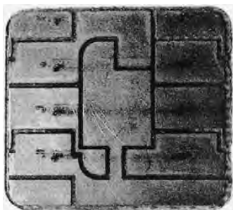
Figure 15.1 Photograph of a module after 50,000 insertion cycles using very high-quality contact elements in a testing machine constructed for this sort of testing. In practice, the contacts may be abraded considerably faster, depending on the type of contact unit used
