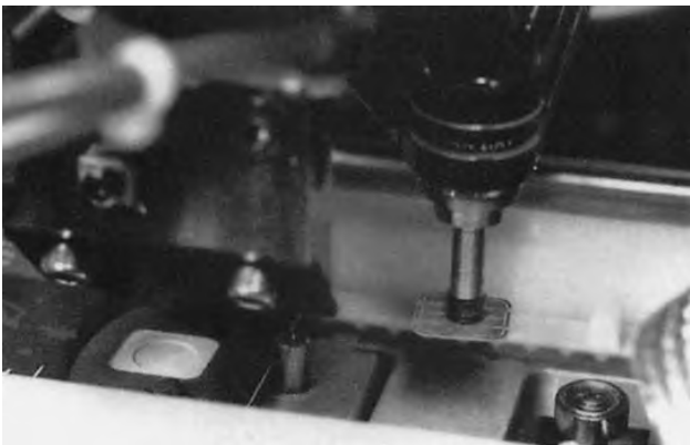
Figure 10.49 Placing a module in the module cavity in an implanting machine (Source: Mühlbauer)
