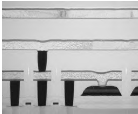
Figure 3.58 Cross-section of a FRAM cell in 0.35- \mu\text{m} technology. The light horizontal bands are aluminum metallization layers, and the dark vertical bars are interconnections ('vias') between the layers. The trapezoidal horizontal area at the lower right is the actual FRAM cell. The width of the cell is approximately 1.5 \mu\text{m} (Source: Fujitsu)
