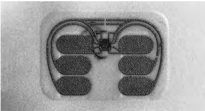
Figure 3.31 A memory chip with an edge length of 0.5 mm (0.25 mm 2 area) and ISO/IEC 7816-3 contact surfaces, fitted to a telephone card along with its contacts using the chip-on-surface process
