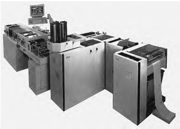
Figure 10.67 A system for attaching cards to their associated letters, which are then stuffed into envelopes along with any necessary attachments. This machine can prepare and stuff up to 7000 envelopes per hour (Source: Böwe Systec)
