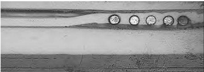
Figure 10.33 Detail of the cross-section of a contactless smart card with an a wound coil embedded in the card body ( Source: Giesecke & Devrient)
