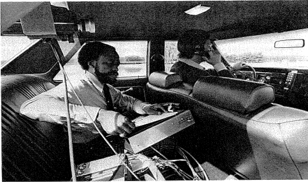
Figure 18-11. Human factors simulation. Laboratory and field simulations play a significant role in the design of user interfaces. Here, human factors engineers use a television camera to study the ease of placing and receiving calls while driving. Tests showed that placing a call with Advanced Mobile Phone Service telephones is as easy as tuning a car radio.
