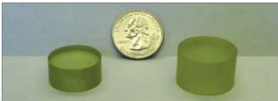
Fig. 1. Cermet has produced these ZnO substrates with a range of dopants to induce self-fluorescence. Eventually, this could lead to the fabrication of high-efficiency, phosphorless white LEDs. With a defect density of only 1 \times 10^4 \text{ cm}^{-2} , the lattice-matched InGaN that has been grown on this ZnO should result in high-performance nitride devices.
