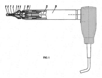
FIG. 1 show an embodiment of a disposable or hygienic module formed according to the invention. A basic module 20 is formed as a conventional handle. The basic module 20 comprises a drive 21 for a needle 3, which is adapted in accordance with the constructive design of a needle shaft 13. ('530 Patent at 3:43-48.)
