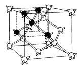
Crystal structure of diamond. Large cube is unit cell. Small cube emphasizes arrangement of bonds between atom at center of tetrahedron and nearest neighbors at vertices.
