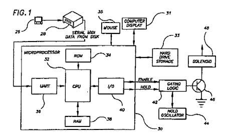
As shown, the Contois system includes a standard personal computer 30 that controls a solenoid 48 that actuates a media playing device such as a player piano. The personal computer 30 in Contois provides a graphical user interface that is displayed to a user on computer display 31. As shown in Fig. 2 (reproduced below), Contois' graphical user interface includes several "panes" of a virtual window, each pane listing music files by category, composer, artist, and song:
