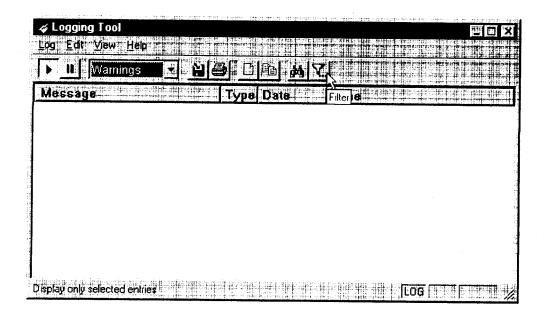
NOTE: The Filter function is an on/off toggle. If the filter is enabled, select Filter Messages to turn it off, then select it again to display the Filter dialog box.
