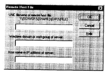
When entering the Universal Naming Convention (UNC) filename of the remote hosts file that you are adding, note that the [SERVER] name is the Windows machine name, not its IP address or hostname.
