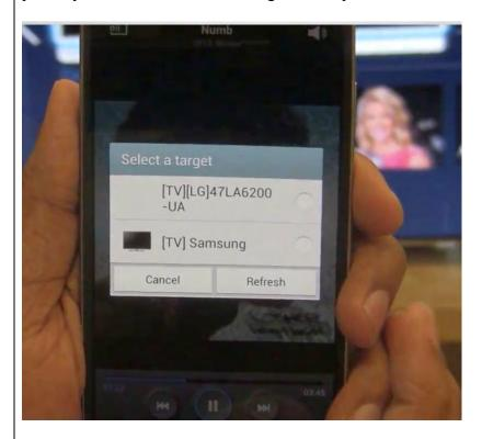
In addition, the picture below shows a representative mobile device displaying a plurality of device identifiers during DIAL operation:
