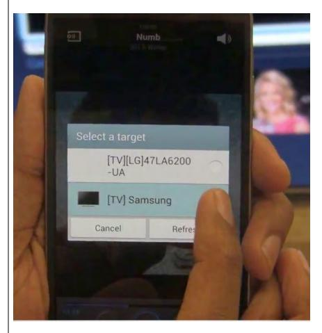
In addition, the picture below shows a representative mobile device selecting via user input at the first device at least one device identifier during DIAL operation:
