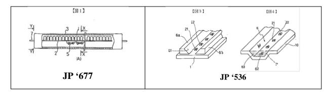
JP '536 discloses that the reflective surfaces bring forward light reflected from the side of each LED, and thereby limit drops in light output immediately above places where no LED is present. Ex. 1010 at Abstract. JP '536 discloses such arrangement providing optical output such that: "output between parts
