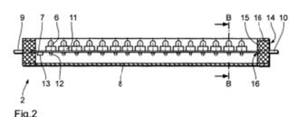
a plurality of light emitting diodes disposed along a length of a bulb portion between a first end cap and a second end cap mounted on opposite ends of the bulb portion, wherein the plurality of light emitting diodes is mounted on only one side of a circuit board in a light emitting direction;
