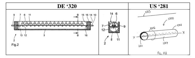
US '281 describes the translucent member 1002 may be implemented in a *substantially cylindrical housing* 1007 provided around LEDs 1001 to provide uniformity of light distribution. US '281 describes:
