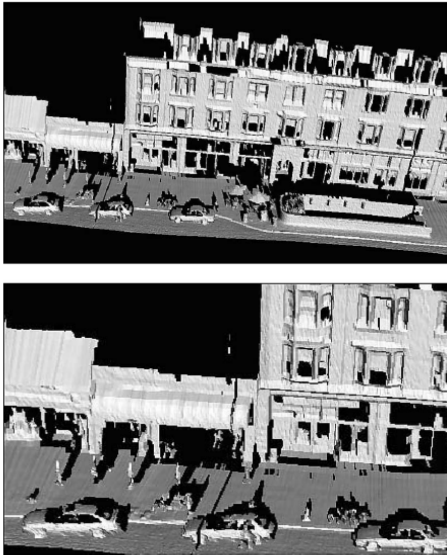
Figure 21. Surface mesh by triangulating the point cloud.
