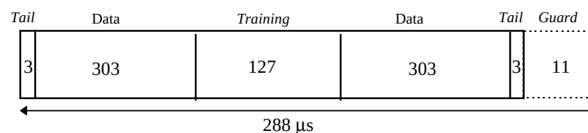
Figure 3-13 The 1/16-slot Synchronisation burst.
