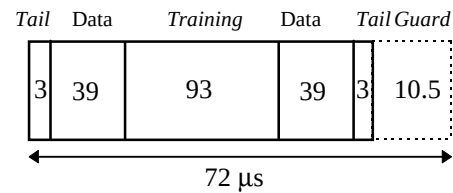
Figure 3-14 The 1/64-slot Synchronisation burst
