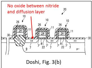
2H. In Doshi, after the diffusion region 7 is exposed by the silicon nitride etch, therefore, a POSITA would have understood that the diffusion region 7, like
