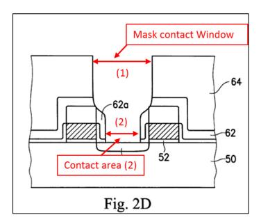
3C. Doshi also discloses a method for forming a self-aligned contact hole. Paper 1, pp. 19-20; Ex. 1003, ¶ A-1. Similar to the '997 patent, the self-aligned contact openings in Doshi are formed using a two-step etch process. Ex. 1005,
