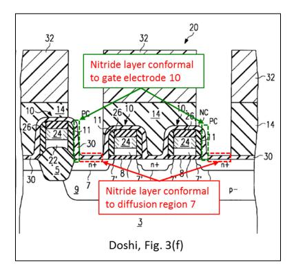
2F. A POSITA would have understood that, if the goal of an etch is to remove the entire nitride layer regardless of direction, an isotropic etch would be
