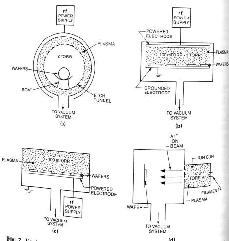
Fig. 2. Equipment used for plasma-assisted etch processes (for simplicity, the manifold used to introduce the etch gases into the system is not shown). (a) Barrel etcher. (b) Planar plasma (or diode) reactor. (c) Reactive ion etcher. (d) Ion milling apparatus.
