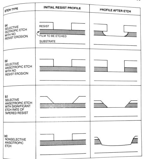
Fig. 1. Etch profiles resulting from plasma-assisted etch processes.
