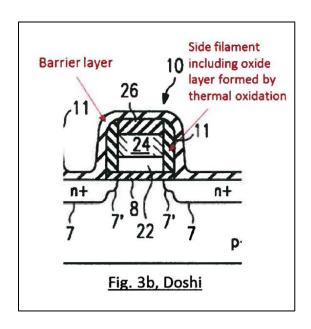
Samsung's argument is based on its incorrect, construction of the term "over" to require only that the oxide layer is higher than the diffusion region, without covering the diffusion region. As discussed in Section IV.B, Samsung's
