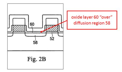
'997 patent at Fig. 2B. As illustrated above, when the '997 patent claims an oxide layer formed over the diffusion region, it is claiming a layer that is actually covering that region, not just higher but off to the side.
