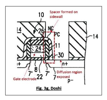
Pet. at p. 27. Samsung identifies this allegedly remaining portion of the nitride layer 30, and calls it a spacer formed of etch barrier material that is formed simultaneously with the etch.
