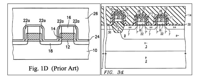
'997 patent at Fig. 1D; Doshi at Fig. 3d. As shown above, the two processes are effectively the same in relevant parts. Both show the thin etch stop layer (layer 24 in the '997 patent; layer 30 in Doshi) formed over the existing spacers (structure 22a in the '997 patent; structure 11 in Doshi) on the side walls of the gate electrode.
