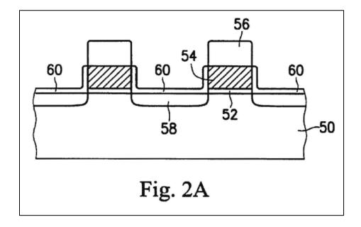
'997 patent at Fig. 2A; 2:55-57 ("[A] thin oxide layer 60 having a thickness of about 150 Å is formed over the substrate surface[.]").
