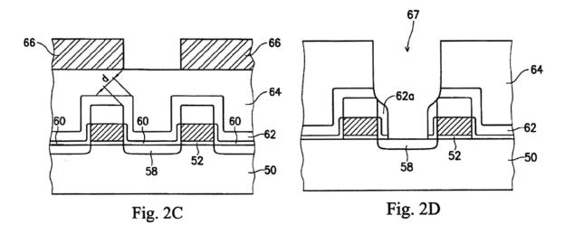
'997 patent, Figs. 2C and 2D. Because the conformal layer is not etched until the contact opening is formed, it also provides extra thickness to protect the gate electrode. *See* '997 patent at Col. 3:32-35.
