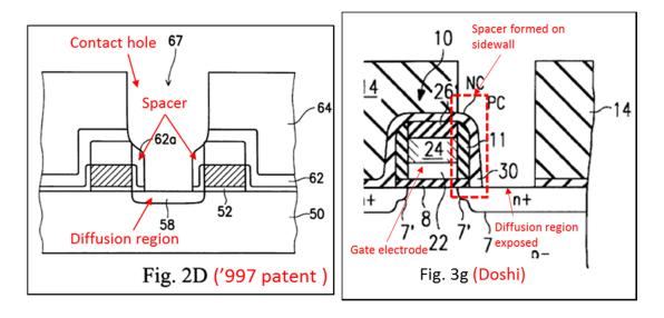
Doshi, in a same manner, discloses a method of fabricating self-aligned contacts. Ex. 1005, Abstract; Ex. 1003, ¶ A-1. In Doshi, after gate electrodes 10, diffusion regions 7/7', gate oxides 8, and sidewall filaments 11 have been formed on a substrate 2, a conformal layer of nitride layer 30 is deposited, followed by a
