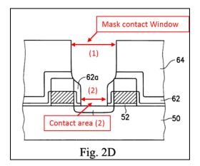
In much the same way as described in Section(III)(A), the process used by Doshi to form its self-aligned contact hole involves a first selective etch and a second highly anisotropic etch. Paper 1, pp. 19-20; Ex. 1003, ¶¶ A-1 and A-12; Ex. 1005, Fig. 3f, Abstract and col. 9:25 – 10:16; Ex. 1011, ¶ 3C. Comparing the
