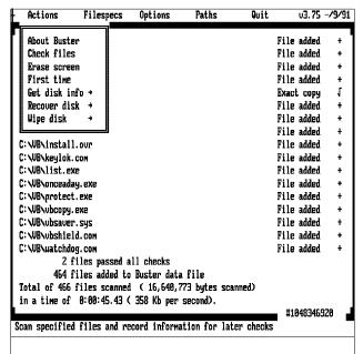
Buster, Leprechaun Software's checksumming program indicating the installation of new files which have not yet been checksummed. The program searches for unknown files. Notice the 'EXACT COPY' diagnosis indicating a checksum match.
