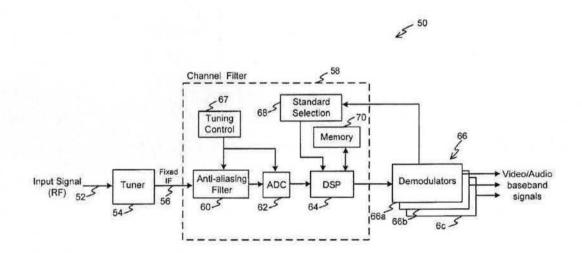
53. The '792 patent, which was filed on July 1, 2004, relates to a television receiver that includes a frequency conversion circuit that receives an input RF signal in one of several television signal formats and converts it to an IF Signal, an ADC that generates a digital
