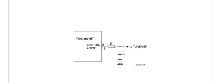
R and C are chosen to verify  $\frac{SR}{1024}$  < f<sub>c</sub> <  $\frac{XIN}{16}$  with R = 1.5 k $\Omega$  and C = 1 nF, f<sub>c</sub> = 100 kHz.
