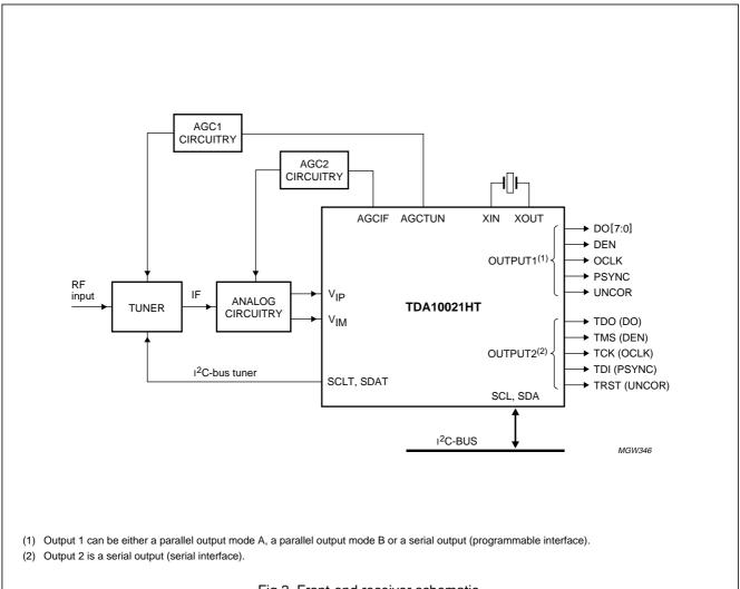
Fig.2 Front-end receiver schematic.
