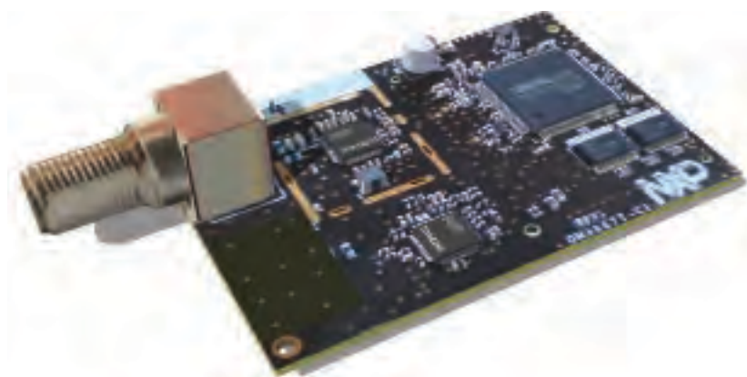
Figure 1 This NXP silicon-tuner evaluation board has provisions for shielding a metal can around the chip, but some applications may not require the can.
