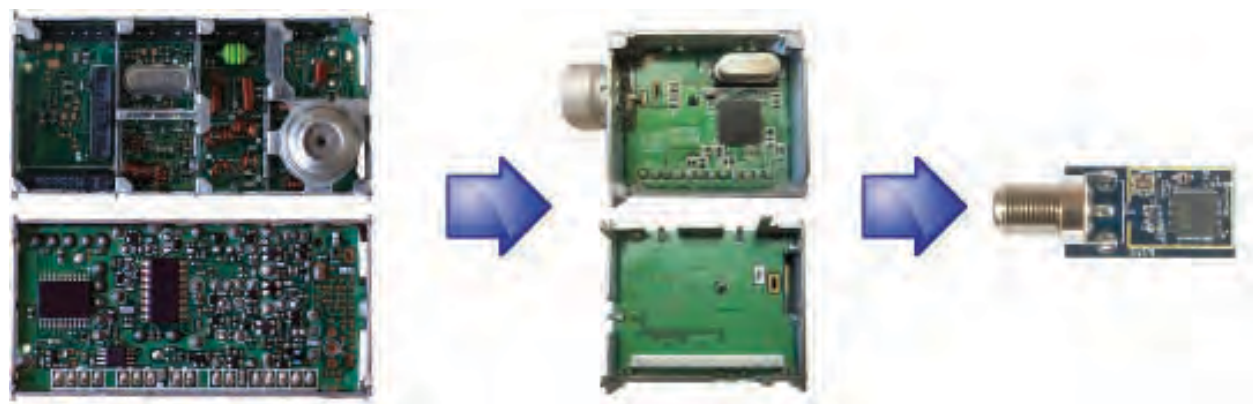
Figure 2 TV tuners are migrating from can-tuner modules (left) toward integrated silicon tuners (center) to devices that designers can integrate directly on the motherboard (right) (courtesy Silicon Laboratories).
