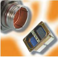
voltage rating of 200 V DC to 120 V ACrms 400 Hz. Current ratings are 15 A, 7.5 A, and 5.0 A for sizes 16, 20, and 22, respectively. The CoF connector is appropriate for high reliability military, aerospace and industrial applications including integrated avionics, radio and navigation systems, fire control devices, electronic counter measures, satellite communications, and data transmitters. Typical pricing ranges from \$125 to \$175 each in quantities of 100.
