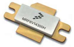
pliant, air-cavity ceramic package, is engineered to manage heat dissipation and reduce heat sink size. The thermal performance provides cooler junction temperature. Other RF performance figures include 330-W peak output power (at 1,400 MHz, 300 ?s pulse width, 12 percent duty cycle), 17 dB gain, and 60 percent drain efficiency.
