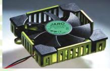
Jaro Thermal's 52-mm × 52-mm × 12-mm Neon fan/ heat sink combination is presented as offering both high performance and low profile. The Neon Series synergistically marries fan to 'open fin' heat sink, and dissipates .275 W/°C. This results in a desirable level of thermal resistance. The Neon Series is designed for semiconductor applications, including FPGA, XPGA, VGA, and most other low profile applications. The life expectancy is 50,000 hours at 25°C. Options include
