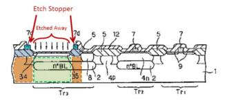
In Fig. 5, the the dummy pattern stops the etch. *Id.* at 46.
