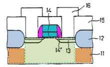
Lee at Fig. 1. The process is completed by depositing a conductive layer **16** into the contact hole to form the contact. *Id.* at 17-2.
