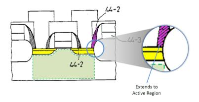
The etch stop layer 44-2 is formed partially on the field oxide layer and partially on the active region, so that it can protect the field oxide layer from damage when etching a contact hole to expose the active region. Lee Decl. at ¶ 122.
