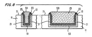
'524 Patent at Fig. 8, 6:6-8. Fig. 8 shows a narrow trench **51** and a wide trench **53**. The '524 Patent further discloses trenches with slanted sidewalls, as a technique known to a POSITA. *Id.* at 7:29-31.
