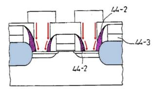
Lee at Fig. 4 (annotated). As shown in Fig. 4, the bottom portion of the contact hole is self-aligned with respect to both the first patterned conductive layer and the etch inhibiting layer, or etch stop layer on the dummy pattern. Lee Decl. at ¶ 128.
