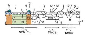
The dummy pattern 7d is "identical" and formed "simultaneously" to the gate electrode 7 on the active region. Yasushige at ¶¶ 31, 41. Both dummy pattern and active gate electrode are made of a conductive material, poly Si film doped with phosphorus. *Id.* at ¶ 44. The dummy pattern is "formed around the base region
