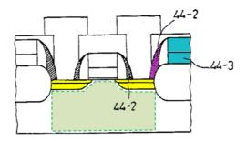
Lee at Fig. 4 (annotated), 17-6. As shown in Fig. 4, the etch inhibiting layer comprises a second patterned conductive layer (44-3), that may be a dummy pattern. Lee Decl. at ¶ 95.
