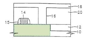
A gate electrode **14** is formed over the active region (green), and spacers **15** are formed along the sidewall. *Id.* at 1:52-56. An insulating layer **20** is formed on the surface of the substrate including the gate electrode **14** and the field oxide layer **12**. *Id.* at 1:56-58. Contact hole **16** is formed by etching insulating layer **20** between
