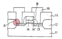
Such damage becomes the cause of junction leakage. *Id.* at 17-2. To address this problem, Lee discloses a method of forming an etch stop layer around the source and drain region by depositing and etching back a spacer having a high etch selectivity **44-2** along the sidewalls of both an active gate and a gate **44-3** on a field oxide layer, as shown in annotated Fig. 4:
