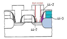
*Id.* at Fig. 4. Lee discloses that the etch stop layers 44-2 are "in the form of a sidewall" and formed using the same process discussed by Lee to form a sidewall on the gate, by deposition and conducting etch-back. *Id.* at 17-5; *see* 17-2 ("forming a gate sidewall (14') using a deposition and etch-back process"). Lee discloses that the gate 44-3 serving as an etch inhibiting layer may be an adjacent internal connection line or a "dummy pattern."
