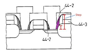
*Id.*; Lee at Fig. 4 (annotated), 17-6. Thus, where the protrusion of the trench isolation layer in the '524 Patent is not sufficient a "step," Lee addresses that issue by providing the dummy pattern **44-3** to form etch stop layer **44-2** along the sidewall. Lee Decl. at ¶ 160.
