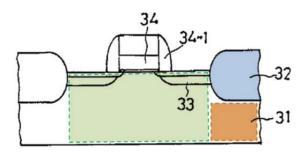
Lee at 17-5, Fig. 3(a). The active region (green) is adjacent the field oxide layer 32 (blue). A POSITA understands that the field region (brown) is then defined by the area of the substrate where field oxide layer 32 is formed. Lee Decl. at ¶ 86.
