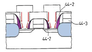
Lee at Fig. 4 (annotated), 17-6. As discussed in Claim 8, the etch stop layer 44-2 is formed with a "material having a high etch selectivity with an interlayer insulation
