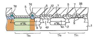
Then, a wet etching process is used to remove the insulating film **12**, as shown in annotated Fig. 5:
