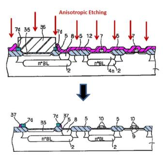
Without the dummy patterns, such over-etching would cause damage to the field oxide region 5, leading to an increase of the leakage current in the substrate. *Id.* at
