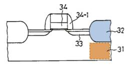
Lee at 17-5, Fig. 3(a). The field oxide layer 32 is on the field region (shaded brown) of the substrate **31** and is a field isolation layer.
