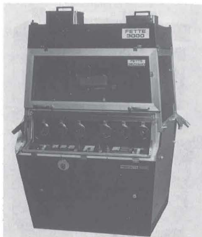
Fig 90-26. Fette Perfecta 3000 high-speed tablet press with pressing compartment completely sealed off from outside environment making cross contamination impossible (courtesy, Raymond Auto).
