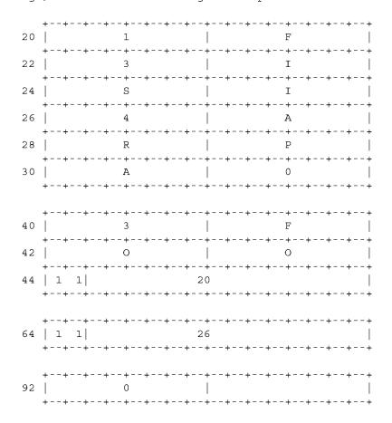
The domain name for F.ISI.ARPA is shown at offset 20. The domain name FOO.F.ISI.ARPA is shown at offset 40; this definition uses a pointer to concatenate a label for FOO to the previously defined F.ISI.ARPA. The domain name ARPA is defined at offset 64 using a pointer to the ARPA component of the name F.ISI.ARPA at 20; note that this pointer relies on ARPA being the last label in the string at 20. The root domain name is
