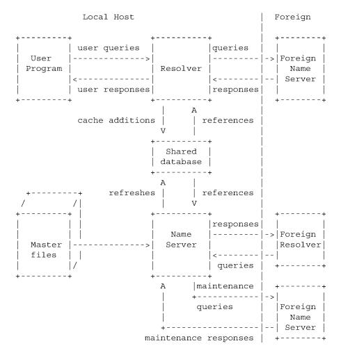
The shared database holds domain space data for the local name server and resolver. The contents of the shared database will typically be a mixture of authoritative data maintained by the periodic refresh operations of the name server and cached data from previous resolver requests. The structure of the domain data and the necessity for synchronization between name servers and resolvers imply the general characteristics of this database, but the actual format is up to the local implementor.
