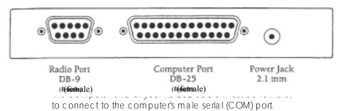
Hint: Since, the KPC-3 Plus's "Computer" port has a female DB-25 connector, the KPC-3 Plus end of your modem cable must have a male DB-25 connector. You also will need to be sure your KPC-3 Plus to computer cable is correctly wired. This topic is covered when we get to the actual installation of the cable.
