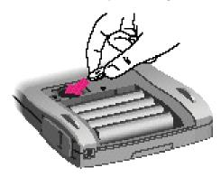
Put back the plate that keeps the backup battery in place. Insert its right end into the slot before you lower the left end (the end with the screw).
