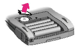
Use a small screwdriver to pry the old backup battery out of its compartment.
