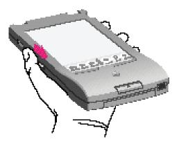
**8** Make sure the MessagePad is turned on. If you don't see anything on the screen, adjust the screen contrast by turning the thumbwheel on the side of the MessagePad.
