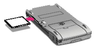
**5** Push the card all the way in to make sure it's connected properly, then lock the card in the slot by pushing the locking tab.
