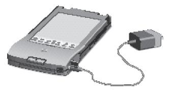
An optional rechargeable battery pack is also available. When the optional battery pack is installed and the power adapter is plugged in, the battery pack recharges.
