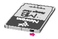
To unlock the card, slide the protection switch back toward the center of the card.
