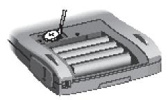
Put in a new Duracell DL2032 3-volt battery or its equivalent. Make sure the battery is + side up.
