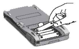
The tab that you pull to remove the batteries should stick out as shown above the topmost battery.
