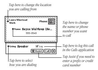
If you want to use a modem to dial, make sure both the modem and the telephone you're using are connected to the same line. See the modem manual for details.
