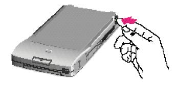
**6** Open the screen lid by pressing in (not down) on the latch at the bottom of the MessagePad and lifting the lid.
