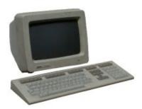
Introduced in 1983. There is no VT200 as such; the **VT220** is a text terminal, while the **VT240** and **VT241** are graphics terminals, supporting Digital's ReGIS graphics and Tektronix vector graphics. The VT240 and VT241 have the same system box; only the monitors are different, the VT240 is black and white and the VT241 is colour. This was the first series to introduce 8-bit communications. They also supported Digital's Multinational Character Set
