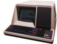
The **VT50** was an uppercase-only subset of the VT52 with only 12 lines. The **VT55** has a primitive graphics capability, somewhat misleadingly referred to as "waveform graphics". It allows the drawing of primitive line or bar graphs. The **VT62** has inverse video mode.
