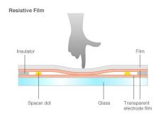
**5-Wire Resistive** Touch is the most widely used touch technology today. A resistive touch screen monitor is composed of a glass panel and a film screen, each covered with a thin metallic layer, separated by a narrow gap. When a user touches the screen, the two metallic layers make contact, resulting in electrical flow. The point of contact is detected by this change in voltage.
