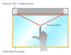
**Infrared** touch screen monitors do not overlay the display with an additional screen or screen sandwich. Instead, infrared monitors use IR emitters and receivers to create an invisible grid of light beams across the screen. This ensures the best possible image quality. When an object interrupts the invisible infrared light beam, the sensors are able to locate the touch point.
