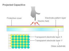
**Projected Capacitive** is similar to Surface Capacitive, but it offers two primary advantages: in addition to a bare finger, it can also be activated with surgical gloves or thin cotton gloves; and it enables multi-touch activation (simultaneous input from two fingers). A projected capacitive is composed of a sheet of glass with
