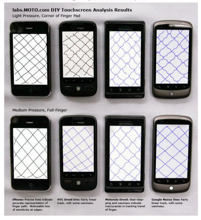
In January, Moto Labs, Moto Development Group's research group, <u>tested</u> <u>different touchscreens</u> by using a drawing program to draw a few straight lines on the display. On a good touchscreen, users can draw clean, straight lines, say the researchers, while inferior touchscreens show lines that look
