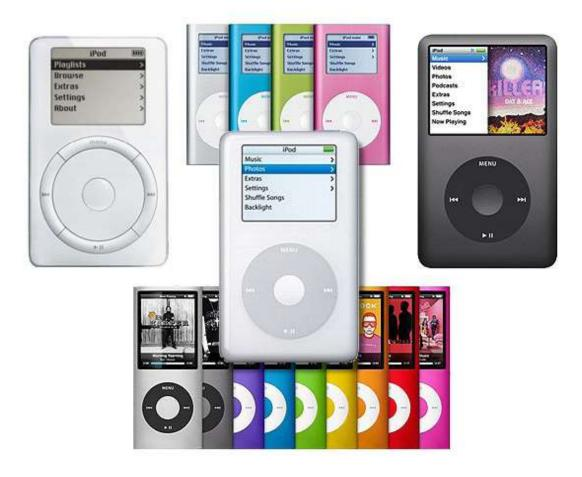
A decade ago Apple introduced the iPod, and with it a new method for controlling music playback: a scroll wheel with buttons around the perimeter. The interface was novel for a portable music player, which usually used more traditional buttons in a linear or grid layout.
