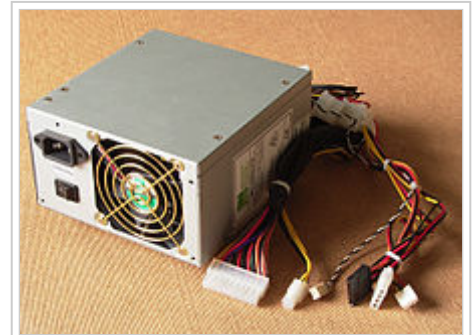
Typical ATX 1.3 power supply. From left to right, the connectors are 20-pin motherboard, 4-pin "P4 connector", fan RPM monitor (note the lack of a power wire), SATA power connector (black), "Molex connector" and floppy connector.
