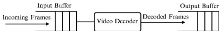
Fig. 7.25 I/O buffering for video decoder: since decoding time varies from frame to frame, the input buffer is needed to hold the frames streaming in. All the decoded frames are buffered into the output buffer until the GOP is completely rendered, and only then the decoded frames of the entire GOP are streamed out
