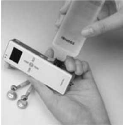
Figure 8.23: Toshiba DMFC-Based MP3 Player
