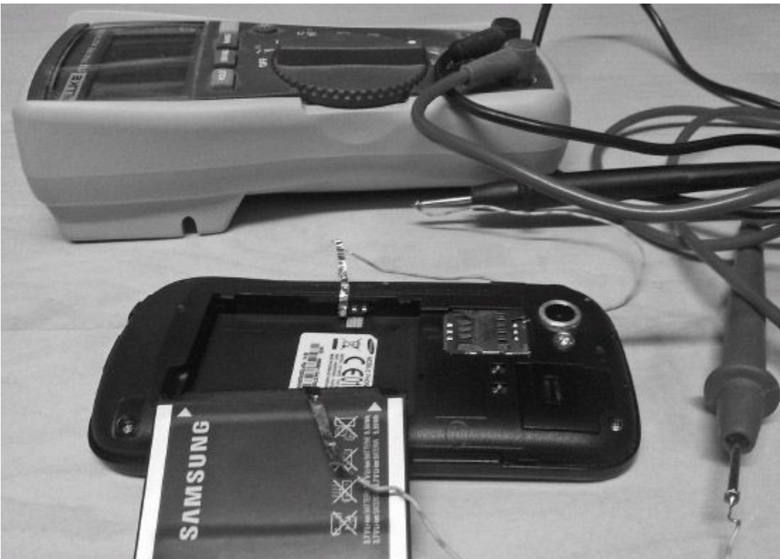
Figure 4.4 The Google Nexus S smartphone with a multimeter connected for measuring current
