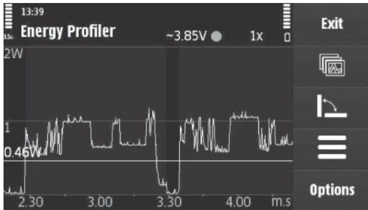
Figure 10.3 Nokia Energy profiler, running on an N97 smartphone, recording estimated power use in watts
