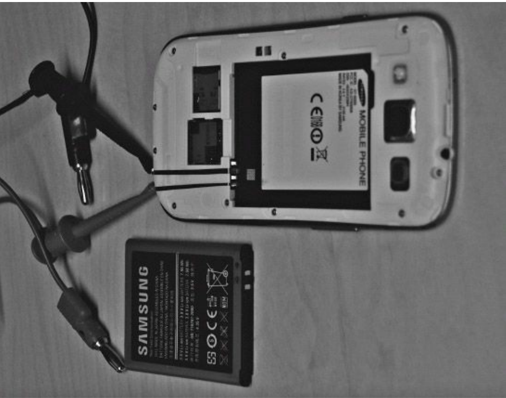
Figure 4.3 A Samsung Galaxy S III ready for hardware power measurement, with battery terminals taped over and phone terminals connected to standard leads with copper tape
