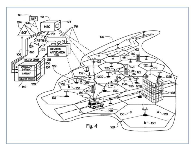
33. Each mobile station is connected to the wireless network through one of the base stations, and the base stations are connected to the public switched telephone network through the mobile switching center. The base stations may either be typical stationary base stations or may be mobile base stations. Mobile
