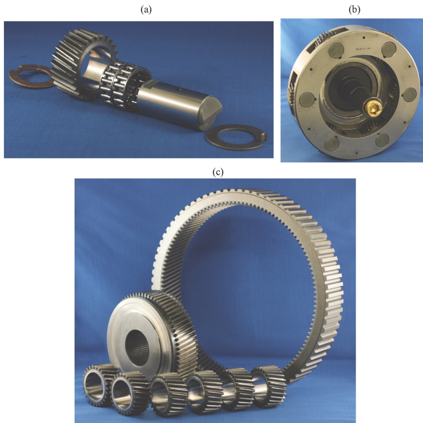
Fig. 3. (a) A test planet gear with its pin, bearings and thrust washers, (b) the carrier assembly, and (c) the gears of the test gear set.
