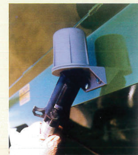
Electrical plug storage receptacle keeps plug clean.
