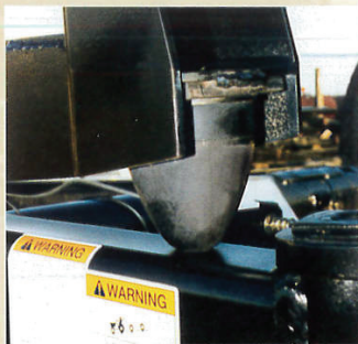
Rubber cushioned rocking bolster provides resilient support and load balance.
