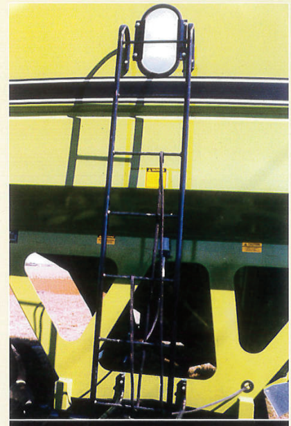
Tubular steel ladder permits safe inside inspection.
