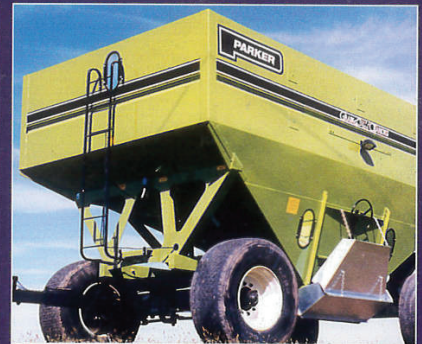
Extra strength end support of one-piece \frac{3}{16} " laser cut plate.
