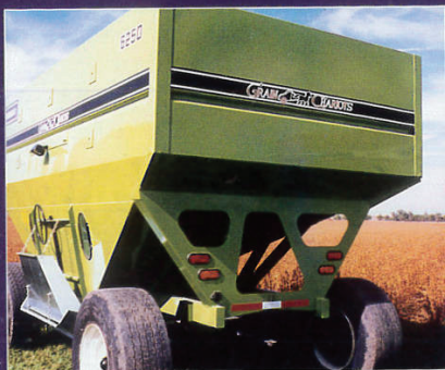
Heavy duty 6" x 3" structural tubing sills offer maximum strength.
