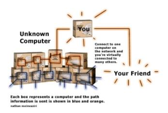
As you can see the box that says, "You" connects to another box or computer. "You" is directly connected to that box and indirectly connected to all of the other boxes. When a search is done, "You" send the search to the box it is directly connected to, and that box sends the search to all the boxes it is connected and so on and so forth.
