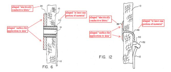
As shown above, each of electrodes 24, 38 has no surface for application to the skin on which tubular connector 22 or conductor 46 is located. Rather, electrodes 24, 38 have a void through which tubular connector 22 and conductor 46 respectively pass to the surfaces of electrodes 24, 38. Indeed, SST appears to
