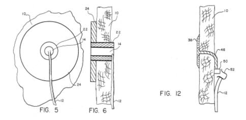
*Granek* further discloses that "[t]he conductors 12, electrodes 24 and 38 and pockets 26 may be metal or conductive cloth." *Id.*, 5:8-9. And "[i]n the conductive embodiment[,] the tubular cylinder 22 and the electrode 24 might be made of metal or silicone rubber." *Id.*, 6:68-7:2.
