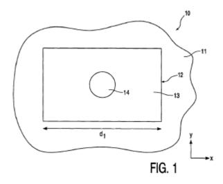
The '951 patent discloses that the electrode arrangement 10 includes "an electrically conductive electrode portion 12 exhibiting a first surface 13 and a portion of material 14 located on the first surface 13." *Id.*, 3:49-53. The portion of material 14 is substantially impermeable to moisture, and in one embodiment, "is of silicon rubber loaded with carbon black." *Id.*, 3:55-58. The electrode portion 12 has a "knitted construction," and in one embodiment, is formed from electrically
