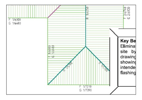
AppliCad at 25 (hereinafter "Flashings Figure"). The roofing materials here are flashings and fall into one of several categories, including ridge caps (designated by an "R"), gutters (designated by a "G"), and fascia (designated by an "F"). *See id.* at 26. The number and length of these flashings are indicated next to the letter designations, *e.g.*, "R 1/5190" is indicative of a single ridge cap with a length of 5190.
